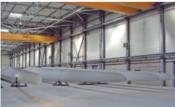
E-Blades Technology S.L. (Spain) Production of rotor blades, adapted to the different VENSYS platform types | Established: 2016
