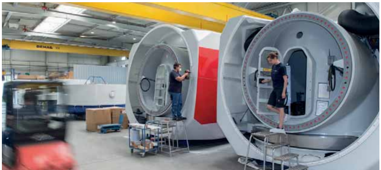
Production of the VENSYS 2.5, 3.0 and 3.5 – 4.1 MW platforms at the company head office in Neunkirchen/ Germany.
