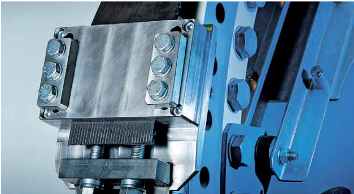
The triple redundant VENSYS blade pitch system is operated via the low-wear and low-maintenance toothed-belt drive.
