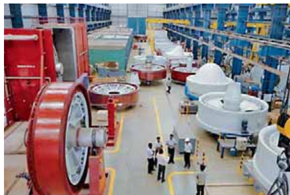
Gearless VENSYS wind turbines are now produced on several continents – shown here is the ReGen facility in India.
